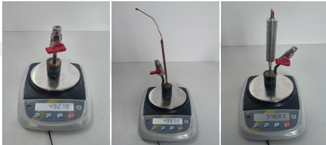
Figure 6.3. Storage tank weights after absorption process is complete.
