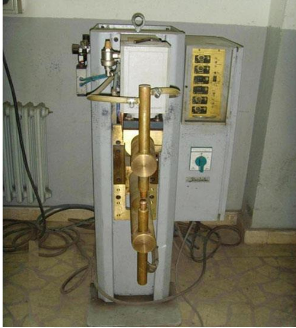
Figure 4.5. Spot welding machine used in this study.
