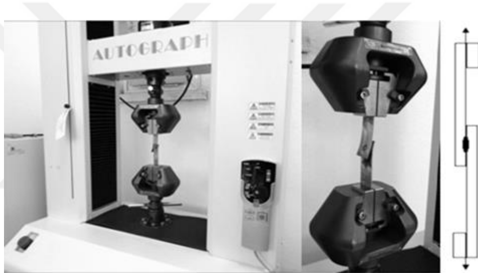
Figure 4.10. Tensile test machine used for testing.
