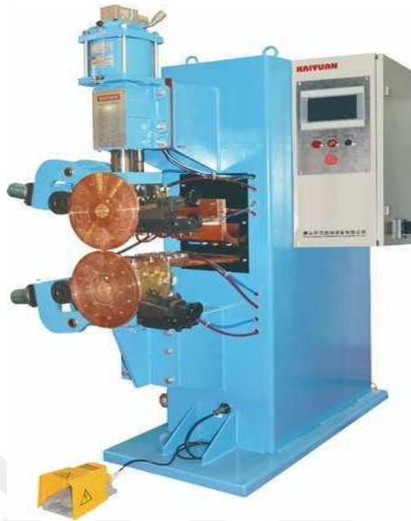
Figure 3.3. Seam welding machine [100].
