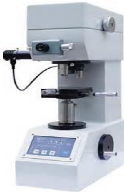
Figure 4.12. The macrograph of Vickers microhardness test machine.
