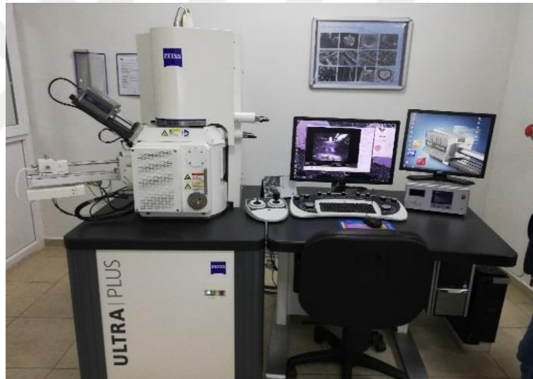
Figure 4.13. The equipment of SEM used for microstructure evaluations.
