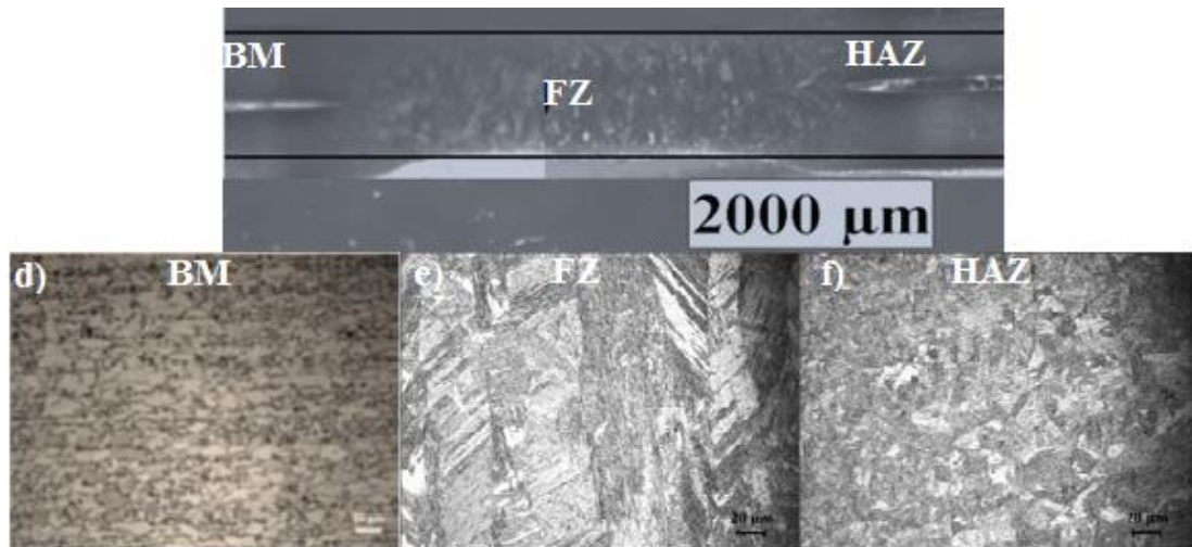
Figure 6.18. The microstructure of weldment joined with 4.5 Bar electrode force with 8kA welding current. d) DP600 base metal (BM), e) DP600 Heat Affect Zone (HAZ), f) DP600 weld nugget (FZ). parameters of (4.5 Bar – 8 kA).
