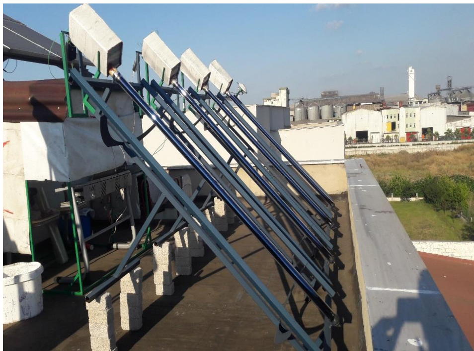
Figure 3.9. Photograph showing the heat pipes receives solar radiation at an angle of 56^\circ .
