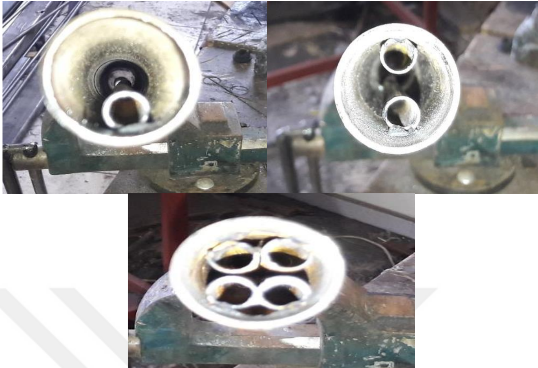
Figure 3.5. Photograph showing internal modifications made on the heat pipe.
