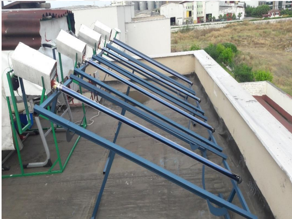
Figure 3.7. Photograph showing the heat pipes receives solar radiation at an angle of 26^\circ .
