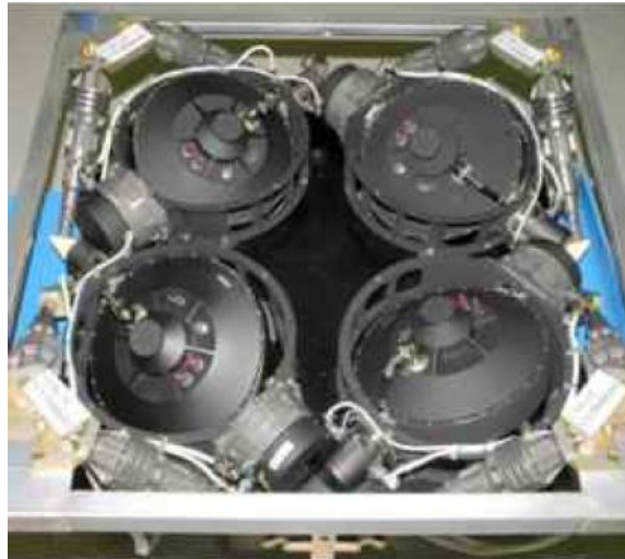
Figure 2.4b. Operational principle CMG [20].
