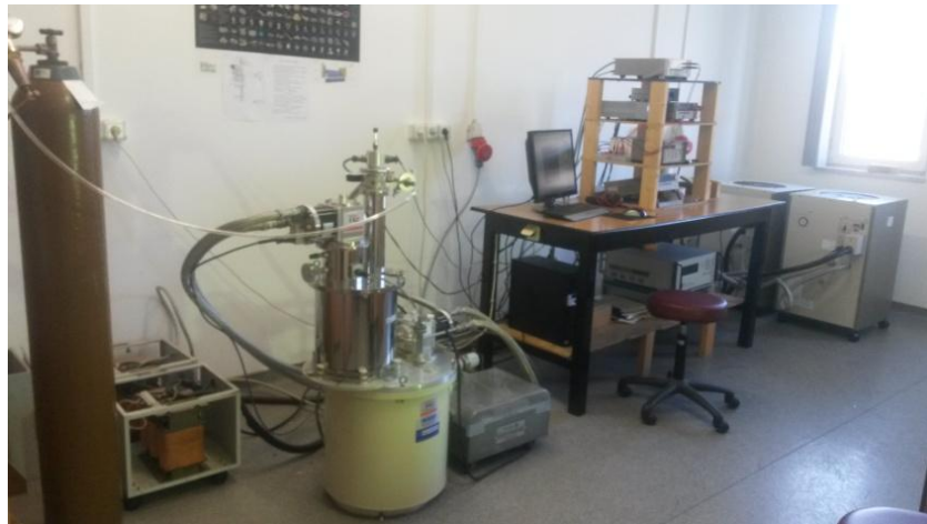
Figure 2.11. He gas closed cycle cryostat system (Cryo Industries).
