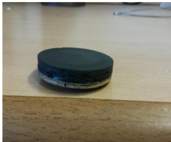
Figure 2.3. Produced Bi-2212 target.
