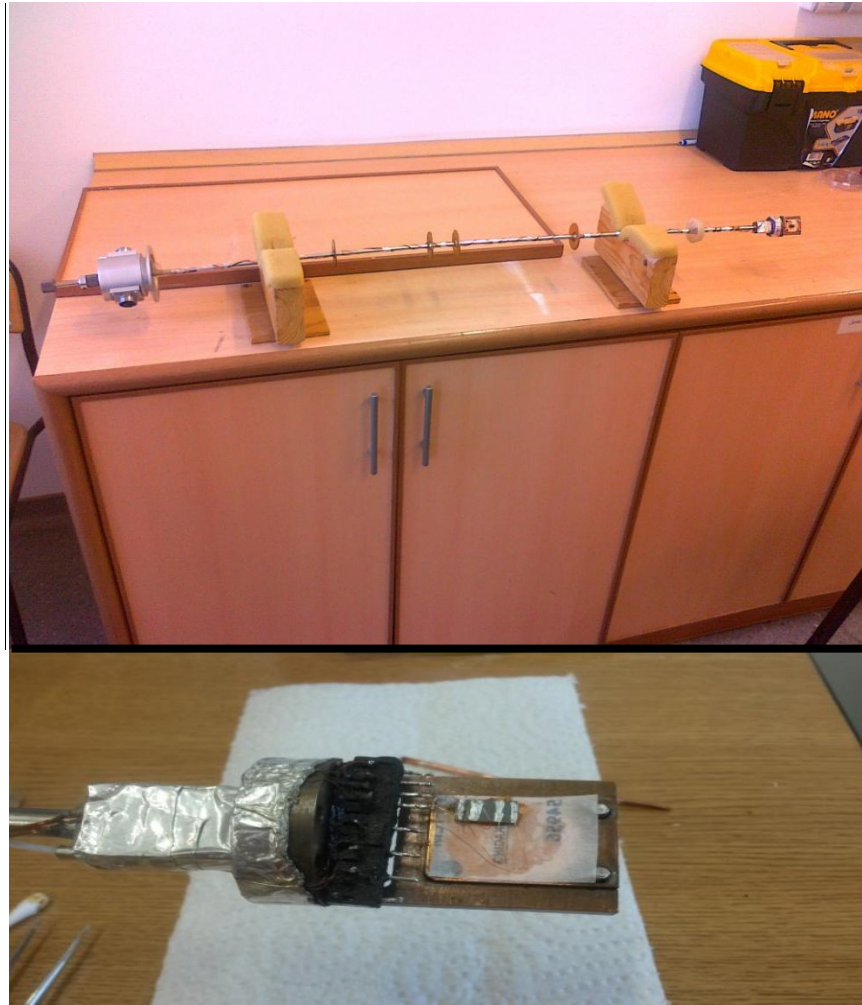
Figure 2.13. Placed thin film on cryostat.
