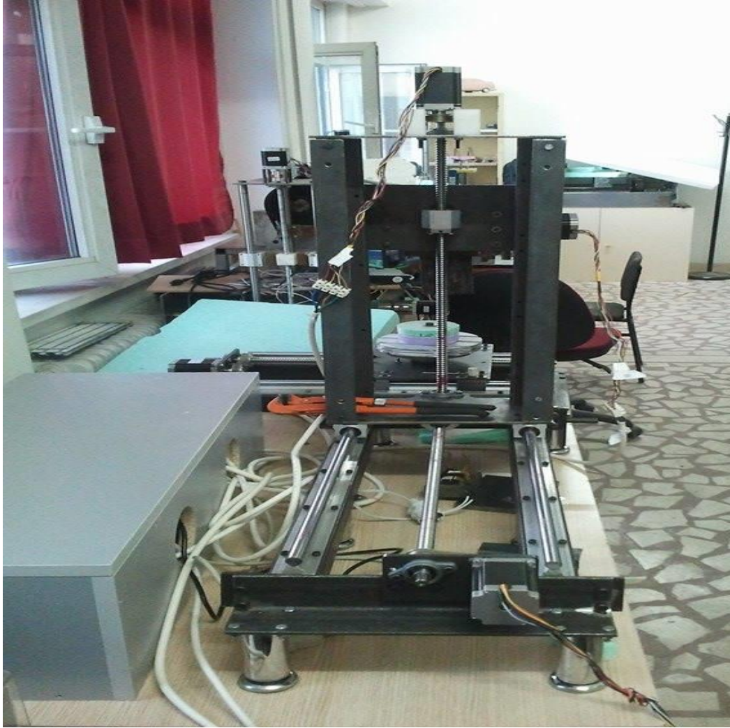
Figure 4.9. Back view of the full constructed 5-axis CNC machine.
