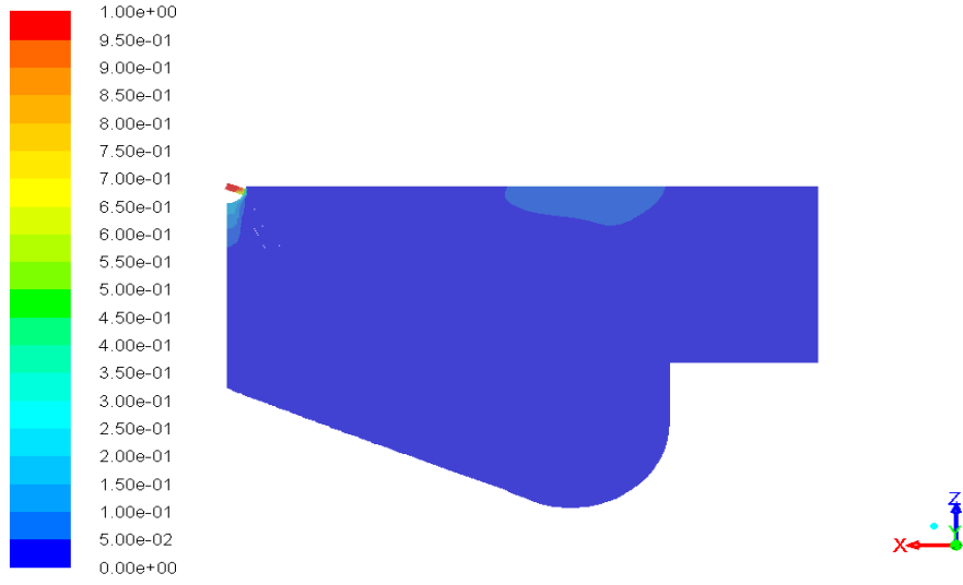
Contours of Mass fraction of ch4 (Time=1.9097e-03) Aug 04, 2015 Crank Angle=750.25(deg) ANSYS Fluent 15.0 (3d, dp, pbns, dynamesh, pdf20, ske, transient)
