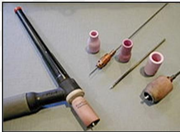
Figure 3.11. Some torches used in GTAW welding.
