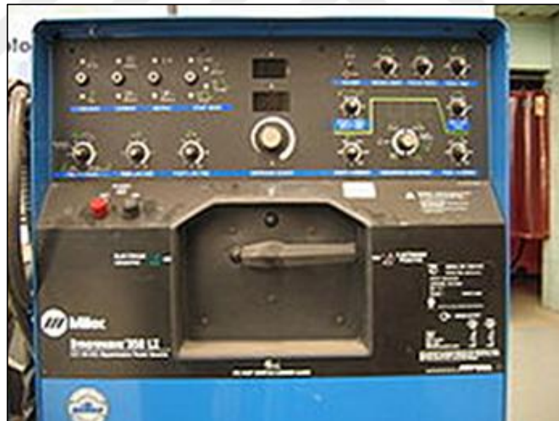
Figure 3.12. Shows a power supply used in GTAW welding.
