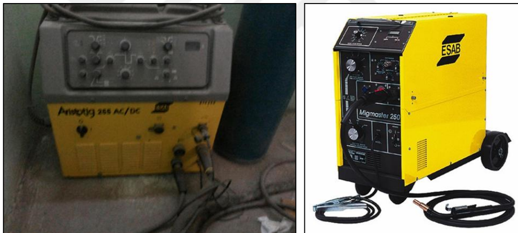
Figure 7.1. TIG and MIG welding machines used.
