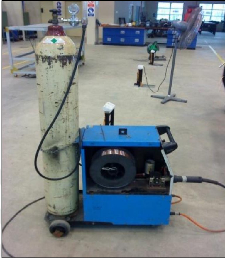
Figure 3.3. MIG welding machine in the welding laboratory.
