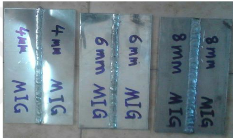
Figure 8.9. Welded samples with MIG welding technique.
