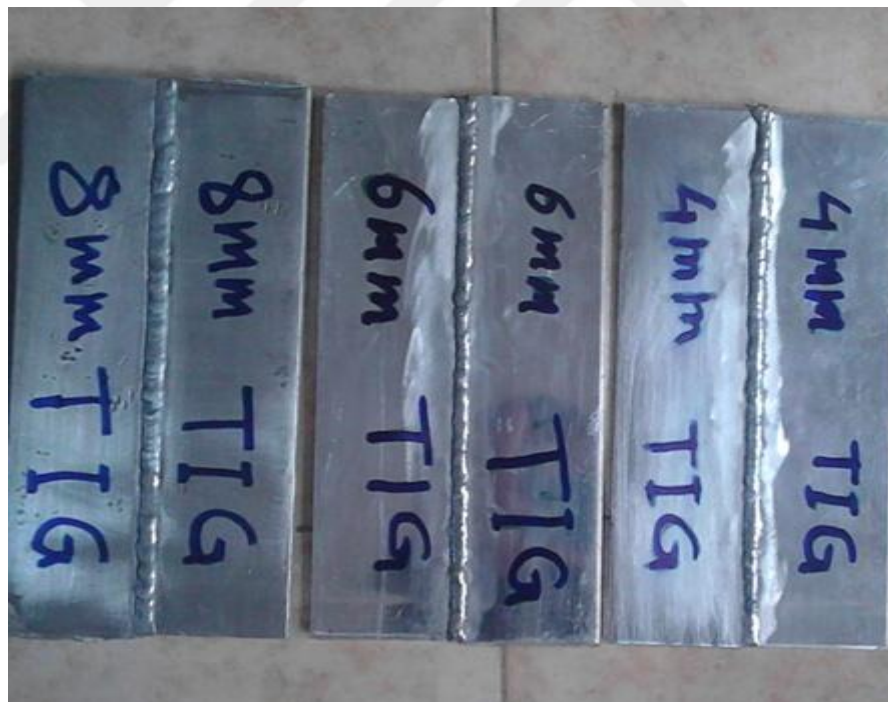
Figure 8.1. Welded samples processed using TIG welding technique.
