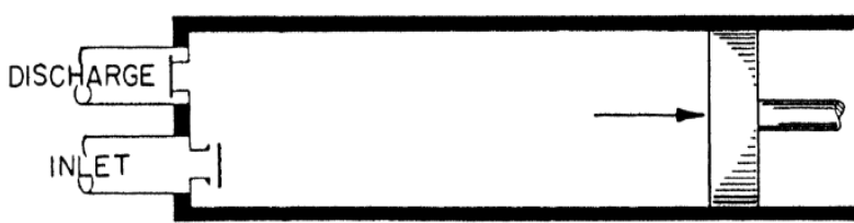
Figure 4.7. Inlet valve open at point 4 and gas flows into cylinder until the point 1 reverse stroke [13].
