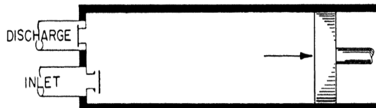
Figure 4.1. A general piston cylinder [13].
