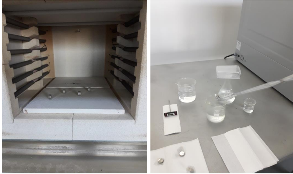
Figure 3.5. The samples image in the furnace quenched into hot water.
