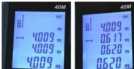
Figure 5.4. Distance measurements between chips and ground with laser meter.
