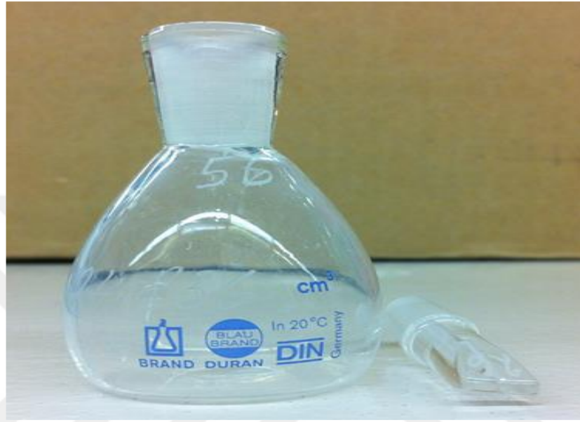
Figure 3.1. Pycnometer used for measuring density of nanofluids.
