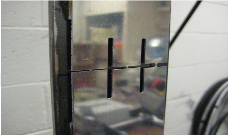
Figure 2.4. Close up of mounted fatigue sensor [11].
