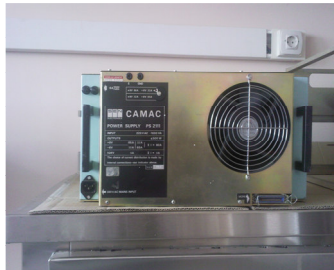
CAMAC Power Supply
