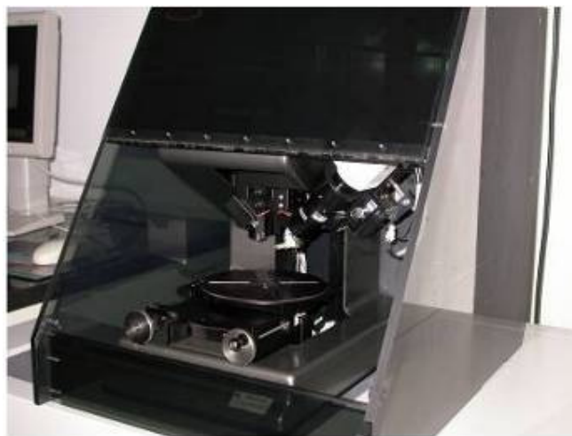
Figure 6.6: Schematic diagram of Veeco Dektak 6M Stylus profilometer [59].
