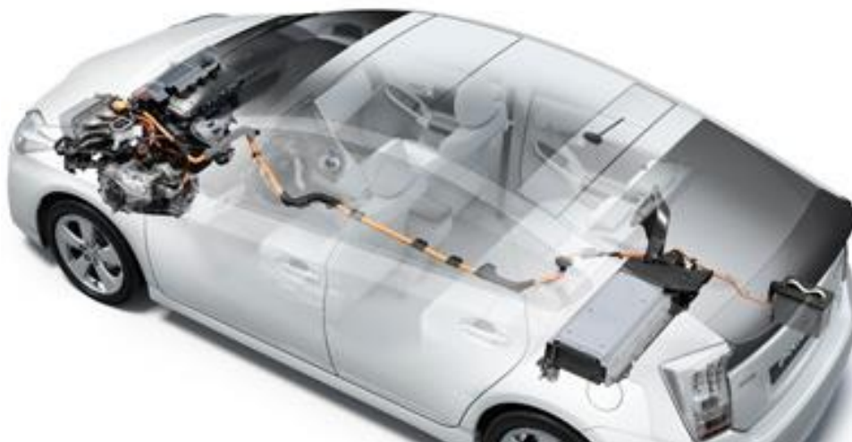
Figure 3.7. Toyota Prius with Series-Parallel HEV Drivetrain (Hobbs, 2014)
