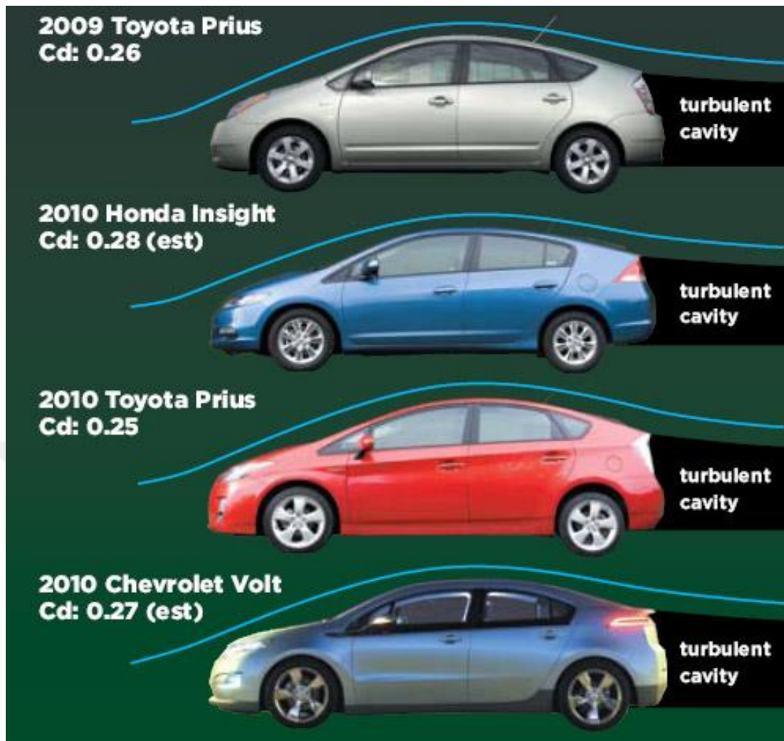
Figure 4.5. Change of Drag Coefficient in Different Designs (Haase, 2009)
