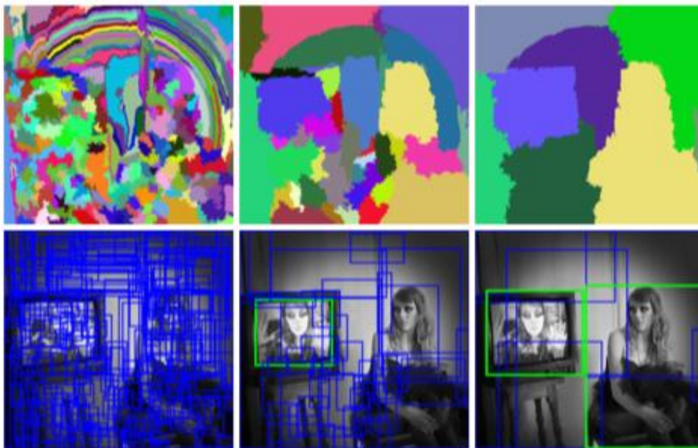
Figure 3.9. The output image after applying Selective Search application
