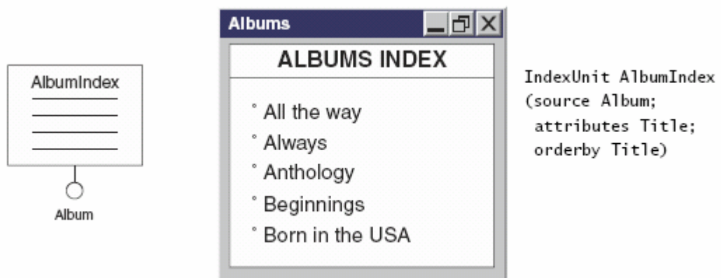
Figure 5.15 WebML graphic notation for index units, rendition in HTML, and a textual definition.
