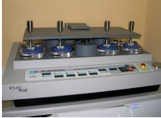
Şekil 9.7.: Martindale Abrasion and Piling Testers, Global Leader in Textile Testing Technologies, Kaynak: SDLATLAS kataloęu, s. 50
