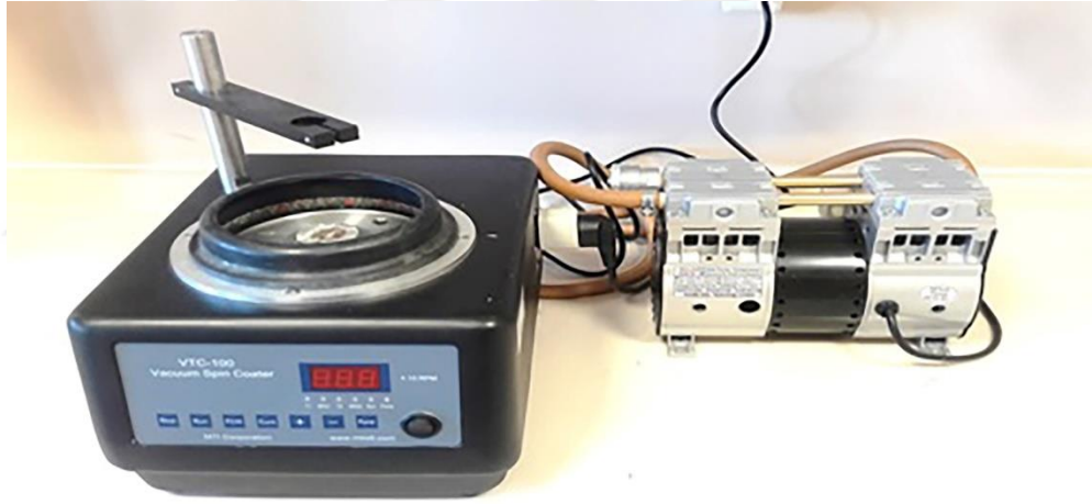
Şekil 3.3. VTC- 100 Vacuum Spin Coater.
