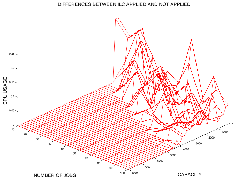
Figure 4.20 CPU Usage Derivations differences when applying Iterative Learning Control and not applying Iterative Learning Control
