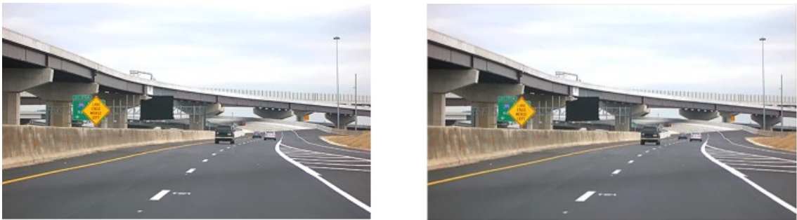
Figure 2.5 : Effect of Gaussian Smoothing Filter : Gaussian filter applied to first image, results the second image.
