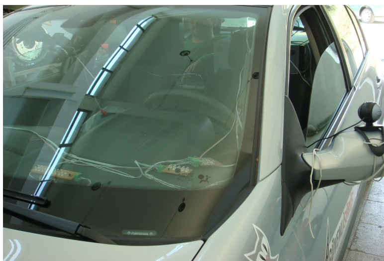
Figure 4.8: Camera Installation on Test Vehicle
