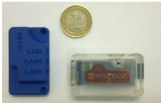
Figure 4.2.1-1 - Shimmer device with ECG board
