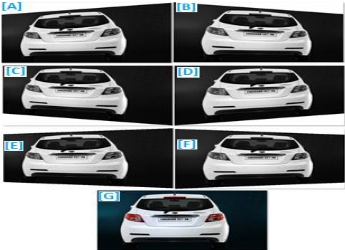
Figure 3.17 - Images A, B, C, D, E, F are perspective planar transformations in different directions of image G. Transformation ratios are [0.9, 0.9] and [1.0, 0.8] .
