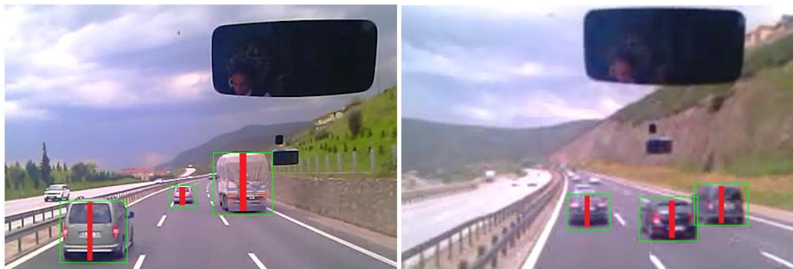
Figure 3.35 - A capture from our recognition and tracking schema on Istanbul TEM Highway
