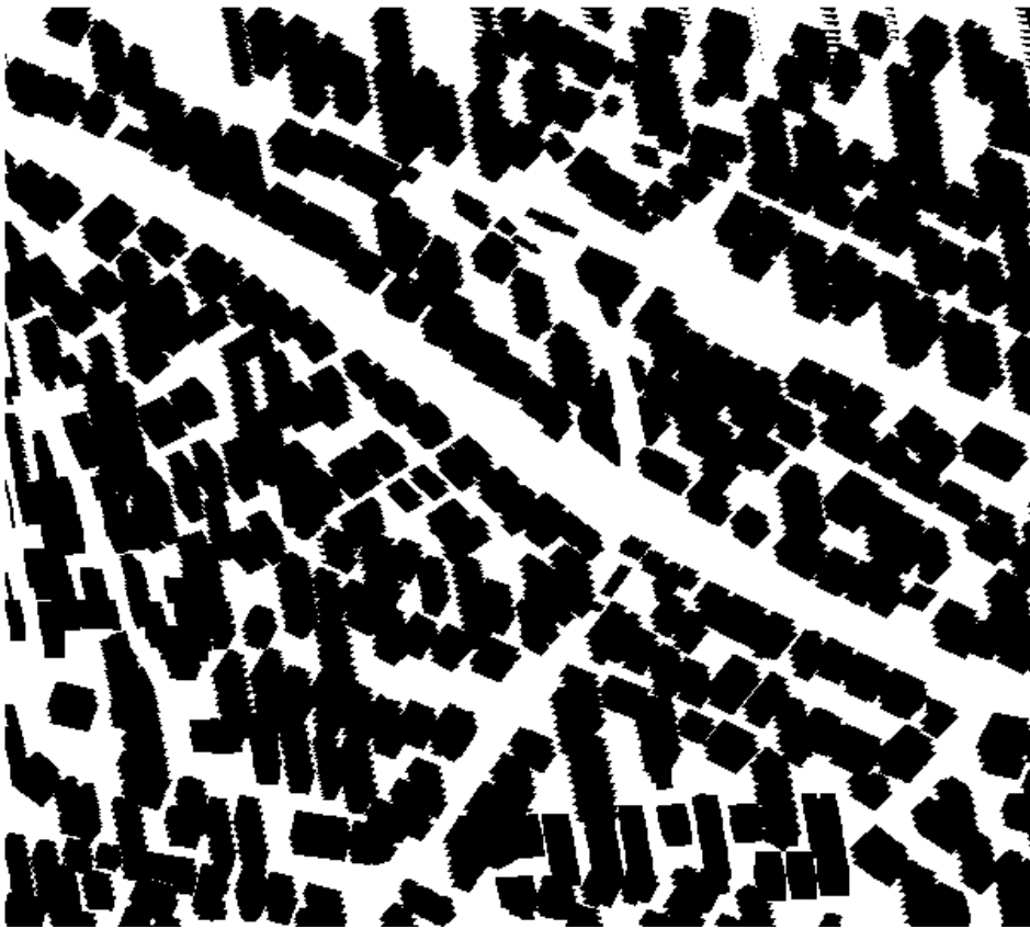
Figure 3.2: Binary occlusion map generated from a single satellite. White areas can see the satellite, black areas can't. Notice the artifacts around shadows caused by limited number of steps used in our algorithm. Increasing the number of steps improves the results.
