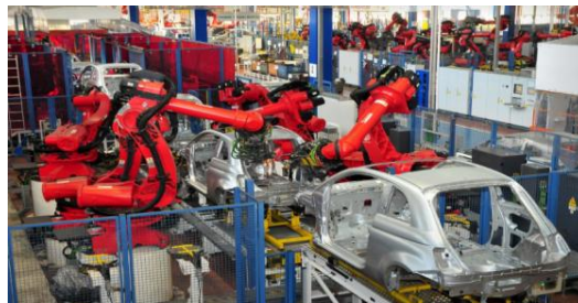
Figure 4.1 A robotic workstation with four robots
