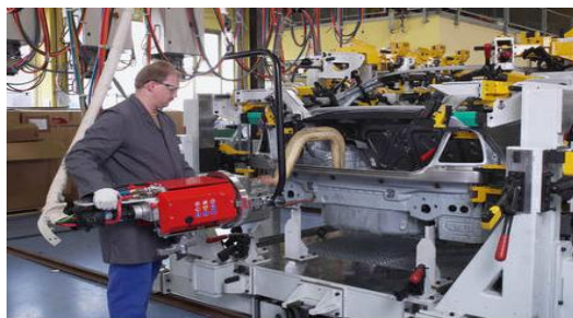
Figure 4.2 A manual workstation with one manual welding gun
