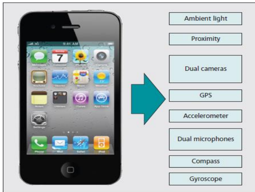
Figure 2.1. An off-the-shelf iPhone 4, representative of the growing class of sensor enabled phones. (Lane et al., 2010)
