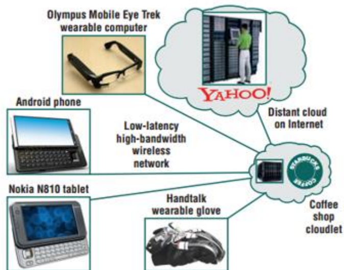
Figure 2.1: The Cloudlet as Proximate Computing Infrastructure Dedicated to the Mobile Devices (Satyanarayanan et al., 2009)
