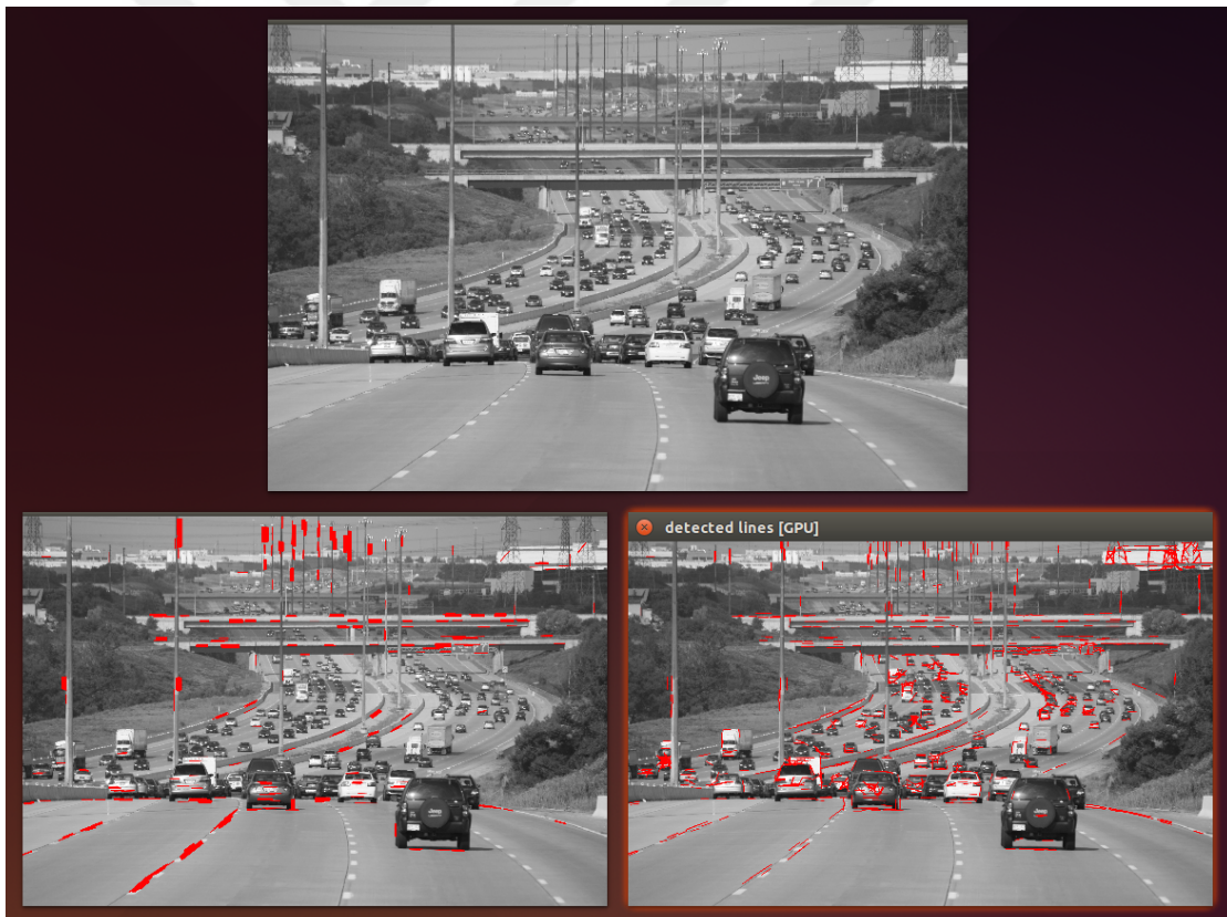
Figure 4.17: Output of CPU vs GPU line detection test on the highway image 3
