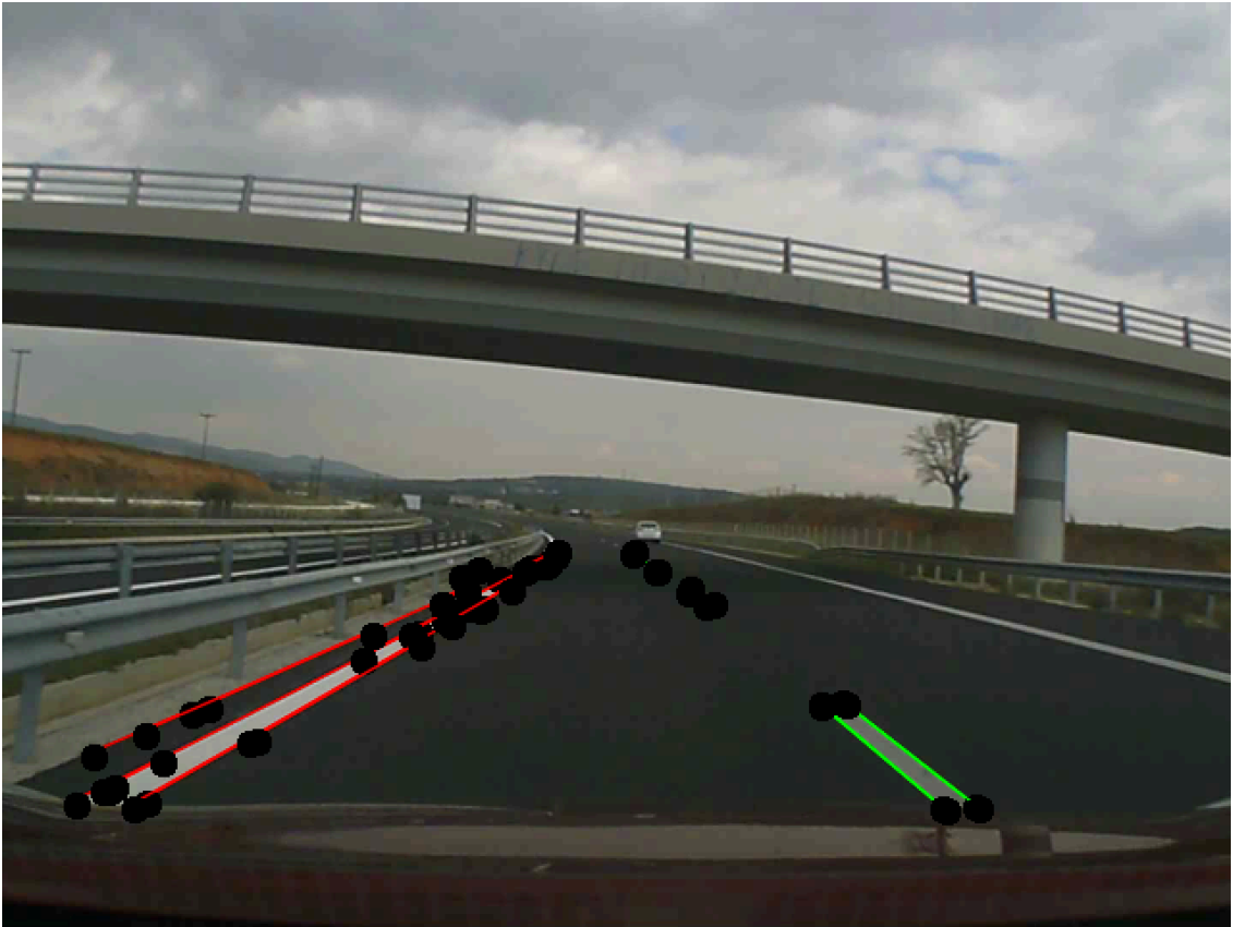
Figure 3.5: Image analysis for the lane marker detection
