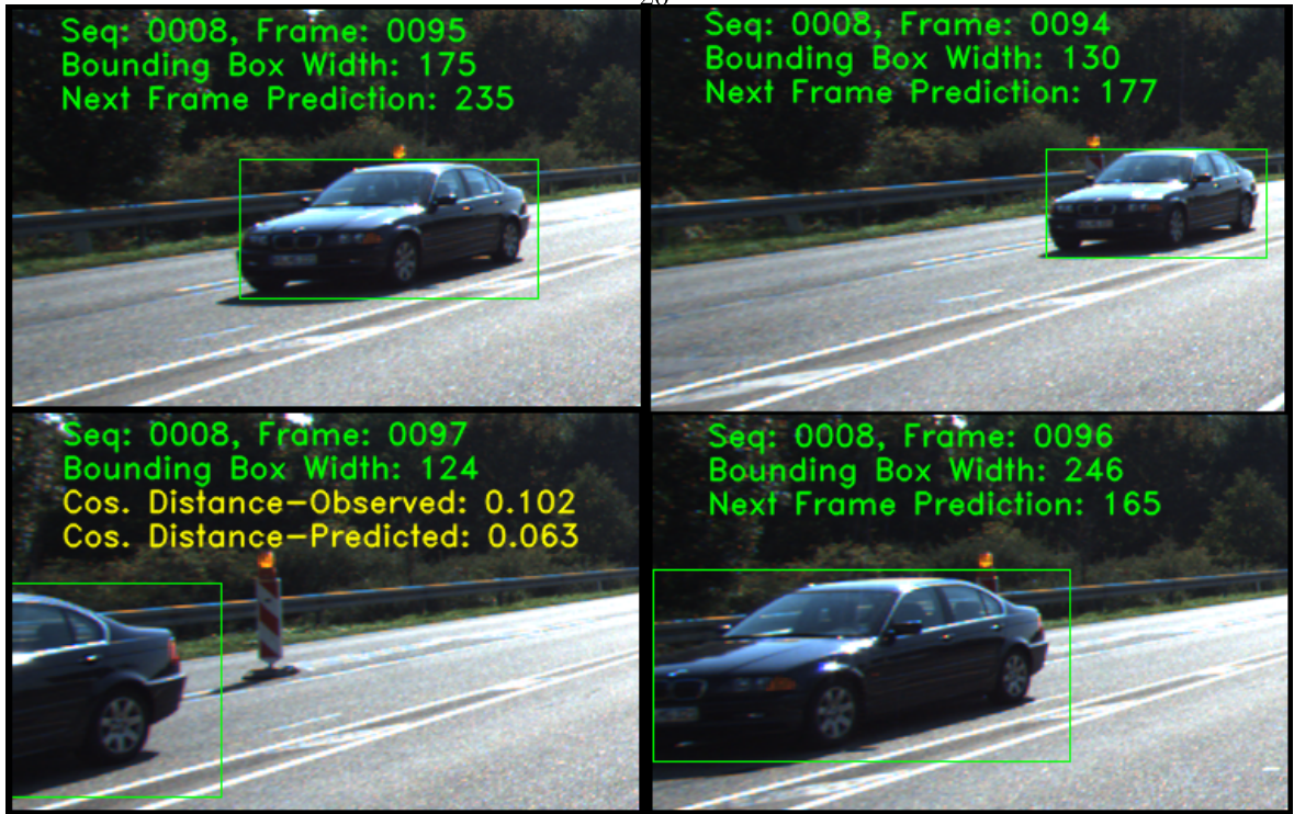
Figure 4.6: The sequence of frames numbered 94 through 97 belonging to Tracking Training Sequence 0008 represents considerable bounding box size changes between consecutive frames. For affinity matching, bounding box of a tracked object that is expected to be partially visible the following frame is adjusted.
