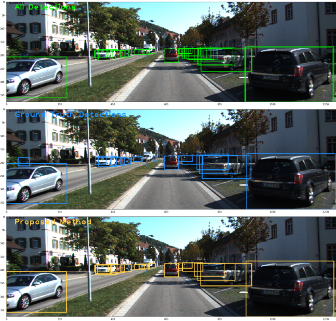
Figure 3.2: Top row shows all 'Car' class detections with confidence higher than 0.05 from convolutional neural network ensemble. Middle row represents the ground-truth bounding boxes provided by the KITTI dataset. Third row is the resulting object bounding boxes from the proposed method.)
