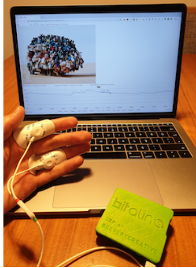
Figure 3.11: Bitalino setup with plugged EDA sensor
