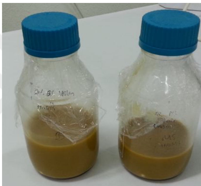
Figure A1.1. Xylan solutions obtained wheat straw (left) and corn stalks (right) from pre-extracted liquor.
