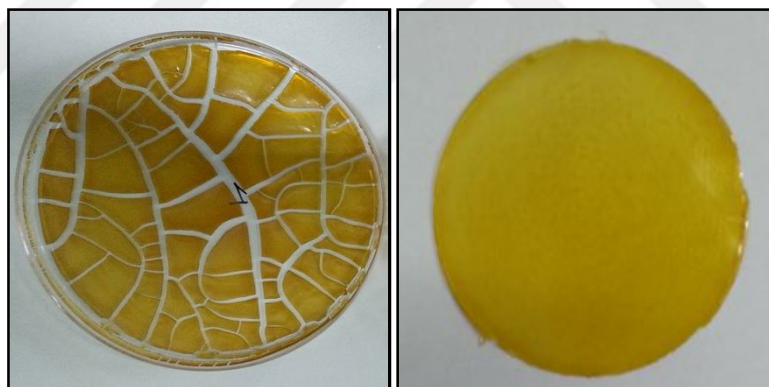
Figure 2.5. Films obtained using only extracted xylan (left) and extracted xylan+xylitol (right).
