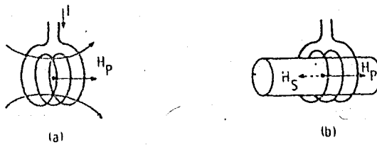
Fig. 2.1 Main principle of the eddy current test:
