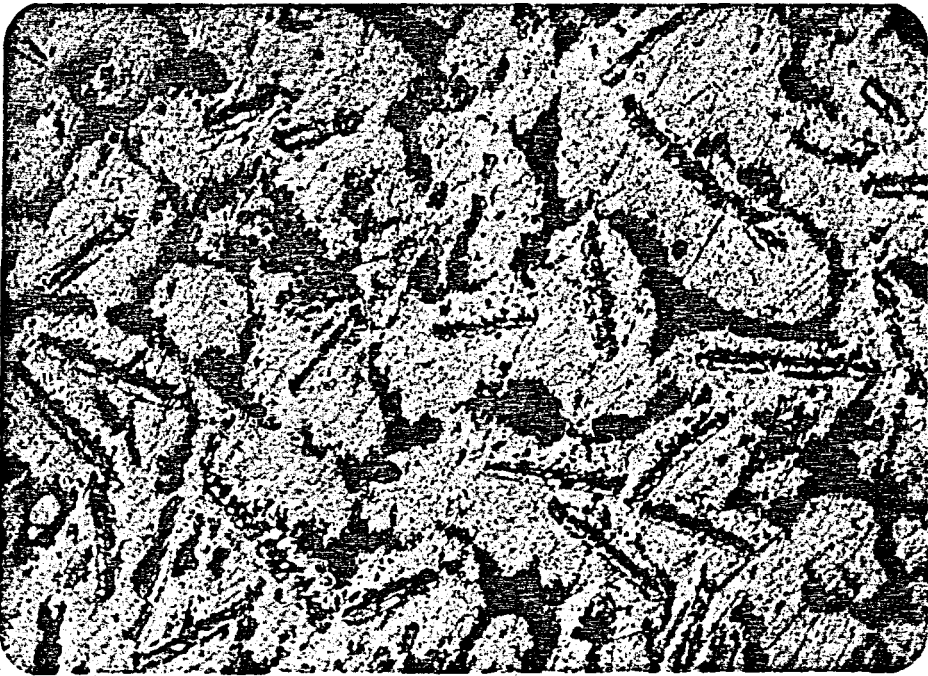
Microstructure of master alloy 16, magnification 165X, 5 min stirring time, 850°C casting temp., Solidification in firebrick.
