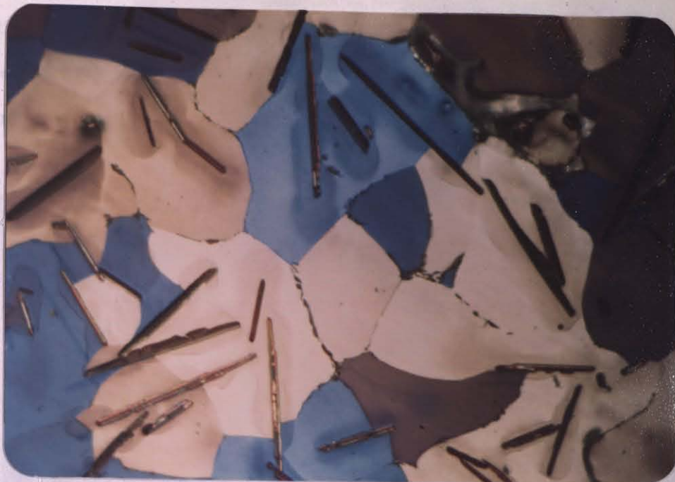
Figure 37- A typical microstructure in master alloy where salts are added at high temperature ( 900^{\circ}\text{C} ). (Etching is performed electrolytically)
