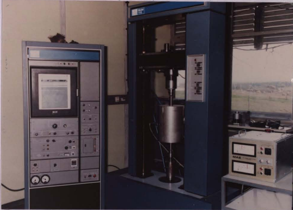
Figure 14 - Instron TT-1115 Universal Testing Machine with Torsion Test Accessory and High Temperature Furnace.
