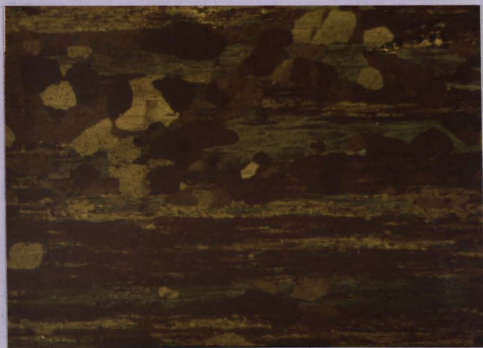
FIGURE 30. Microstructure of the product which was extruded with an extrusion ratio of 25:1 at 400°C initial billet temperature.
