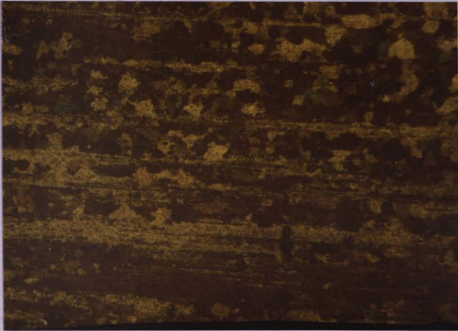
FIGURE 32. Microstructure of product which was extruded with an extrusion ratio of 63:1 at 350°C initial billet temperature.
