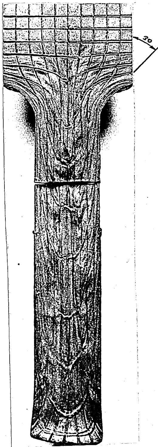
FIGURE 26- Deformed Grid Network of Commercial Lead Alloy after Extrusion.
