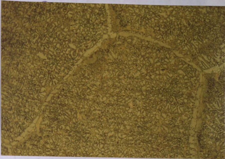
Figure 43 - After hot-rolling at 950°C, etched, incident light. High magnification 250X.
