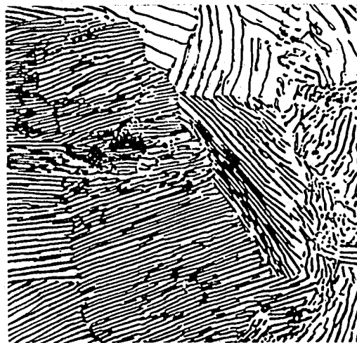
Figure 2. Pearlite in an eutectoid steel (0.77 % carbon, etched by 4 % nital, 1000x) (24).
