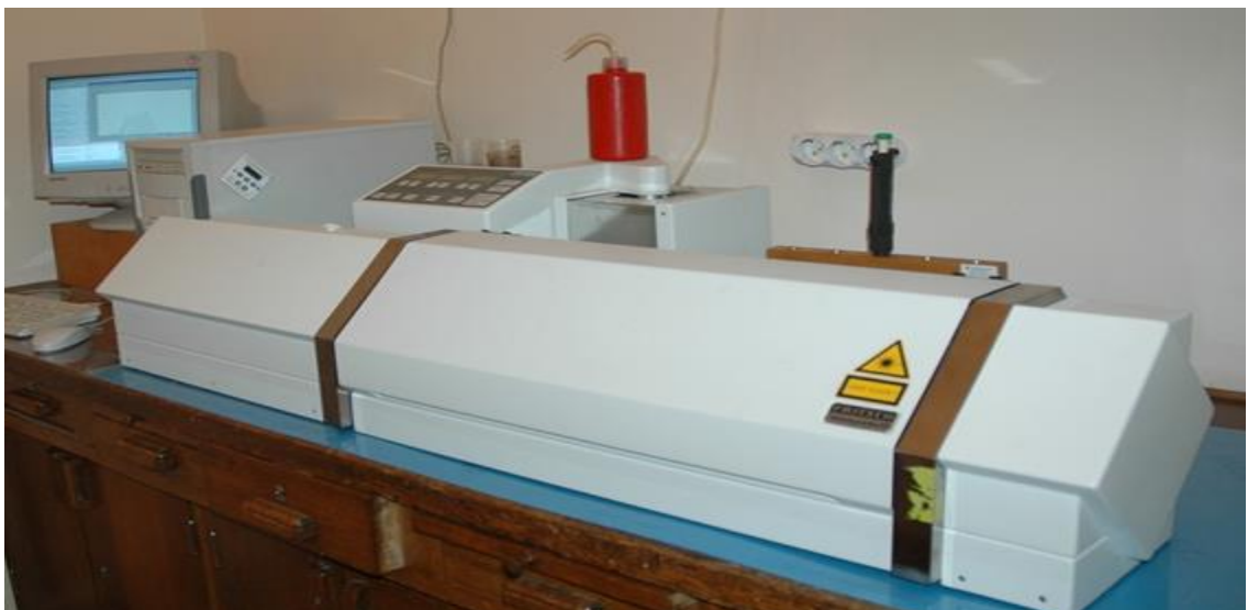
Figure 4.12 The Laser Particle Device used to determine soil particle-size distribution (FRITSCH in Analyset 22 Comfort)
