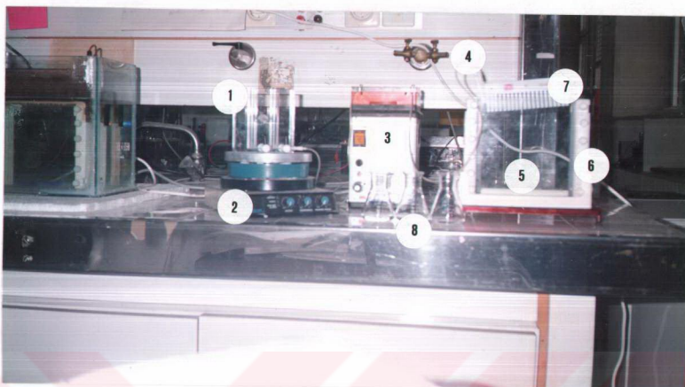
Figure IV.1. Denaturing gradient gel apparatus. 1. Gradient maker, 2. Magnetic stirrer, 3. Peristaltic pump, 4. Thin plastic tube with a needle at its end, 5. Glass plates, 6. Gel frame, 7. Comb, 8. Prepared gel solutions.
