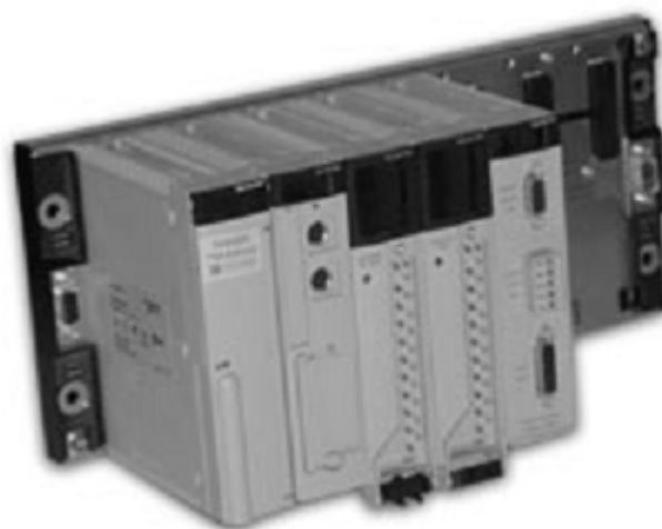
Figure 4.9 – Modicon Premium PLC with its rack
