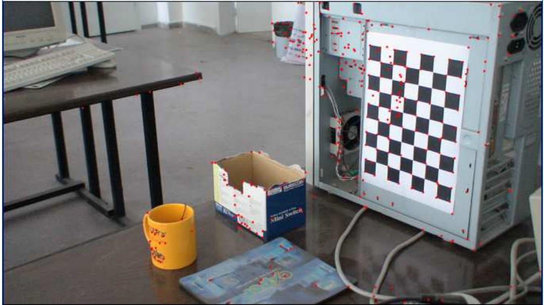
Figure 7.5 : Projection of the 3D corner point coordinates.
