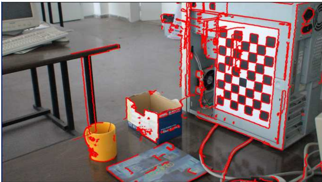
Figure 7.4 : Projection of the 3D edge point coordinates.
