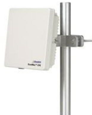
Figure 5.7: Outdoor NLOS (Non-Line-of-Sight) CPE
