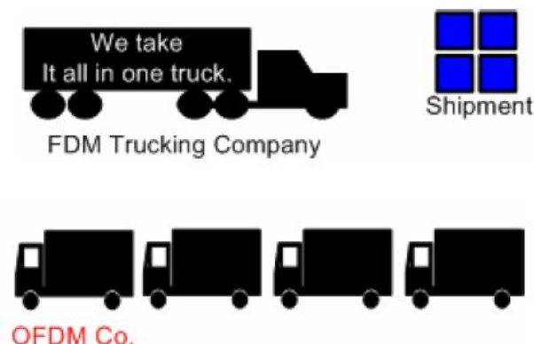
Figure 2.6: A regular FDM and Orthogonal FDM - Example 2: All cargo in one truck versus splitting the shipment into more than one.
