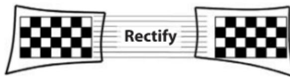
**Figure 2.6:** Rectified, Row Aligned Images [6]
