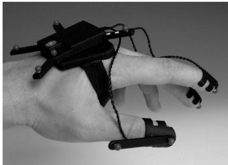
**Figure 2.13:** Transmitters Attached at the Finger Tips [8]
