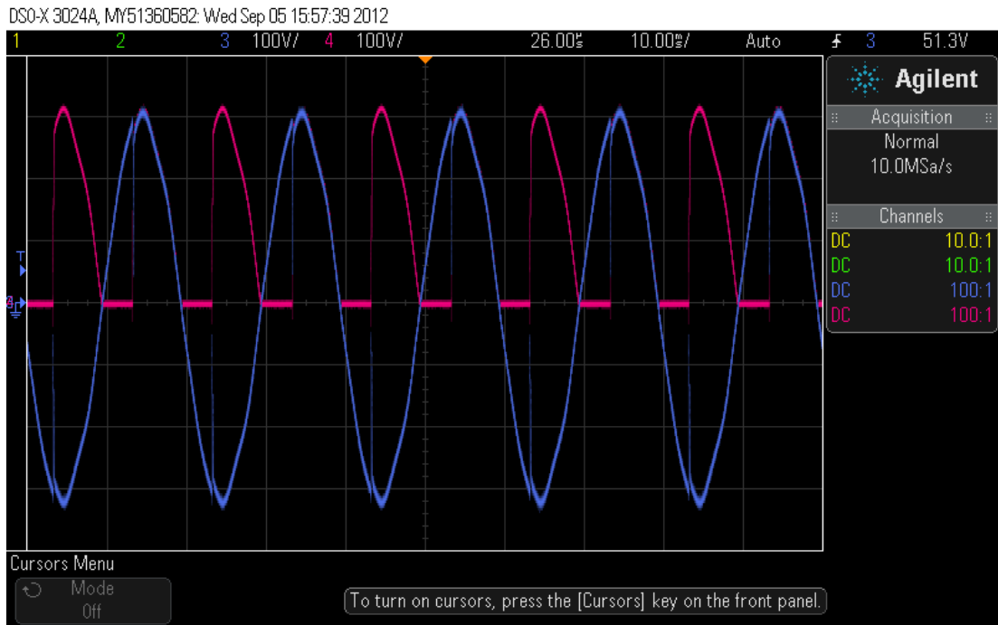
Figure 37: Controllable Single Phase Rectifier Output Voltage Without Capacitor
