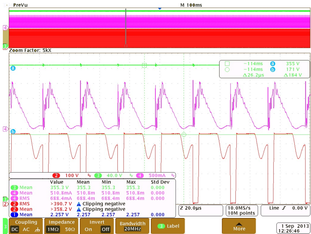
Figure 4.12 Experimental Waveforms of the ZSC. (DCM Operation)
