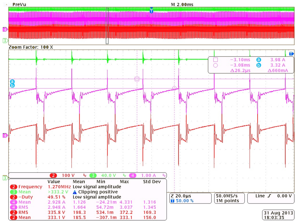
Figure 4.10 Experimental Waveforms of the ZSC. ( I_O, V_{RO}, V_C )
