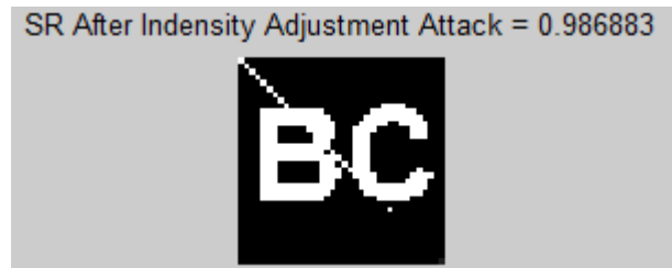
Figure 35. SR value of watermarked image after intensity adjustment attack
