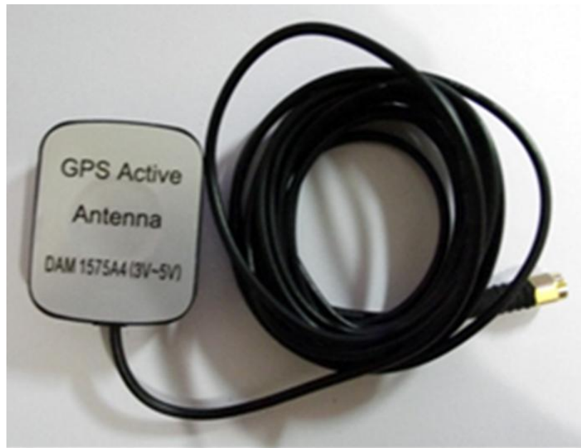
Figure 24. DAM 1575A4 Type Antenna
