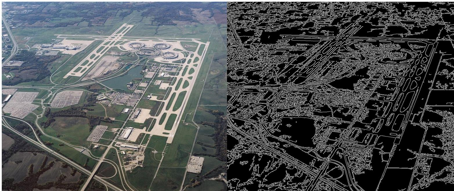
**Figure 49** Example of Canny edge detection
