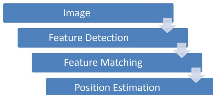
**Figure 1** Visual odometry system
