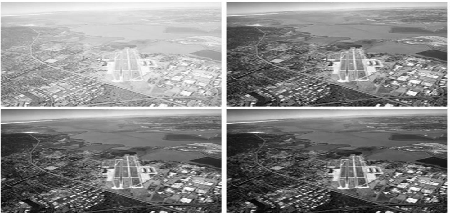
**Figure 41** Example of power-law function application: a) original aerial image, b) result when  $\gamma=3.0$ , c) result when  $\gamma=4.0$ , d) result when  $\gamma=5.0$ , for all  $c=1$
