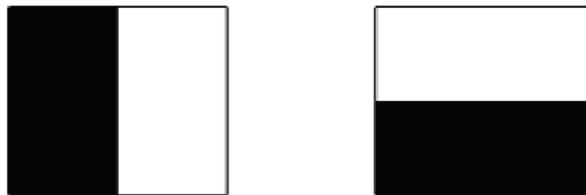
**Figure 71** Haar wavelet filters employed to compute the responses in the x and y directions.
