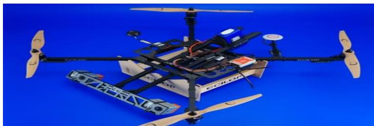
**Figure 77** Project hardware (quadcopter with two cameras)
