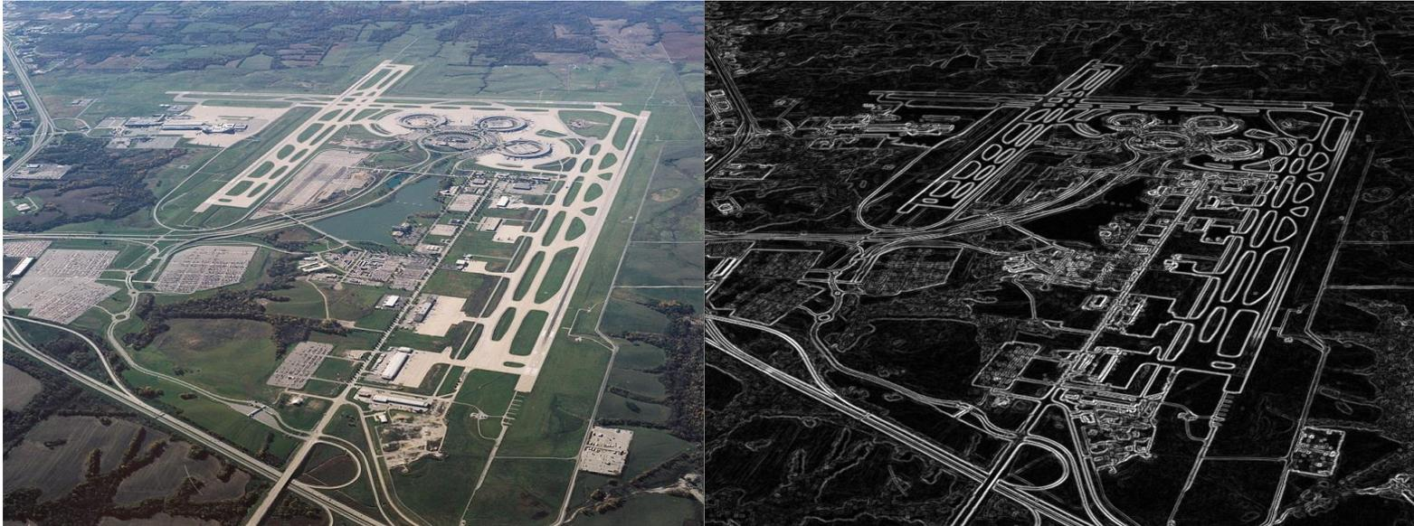
**Figure 51** Example of Sobel edge detection
