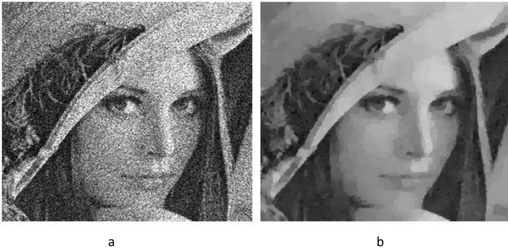
**Figure 44** Mean filter applied to an image: a) image with noise, b) image after mean filtering
